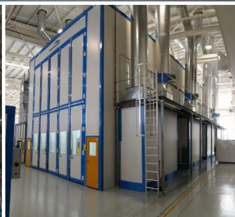
Above: Multiple views of the large scale downdraft facility showing the booth, mechanical ductwork, service platforms and internals.
