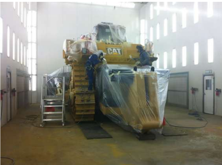
Above: The facility at Caterpillar is about scale and productivity - this large spray booth provides a safe and compliant area for operators to coat cat products.
